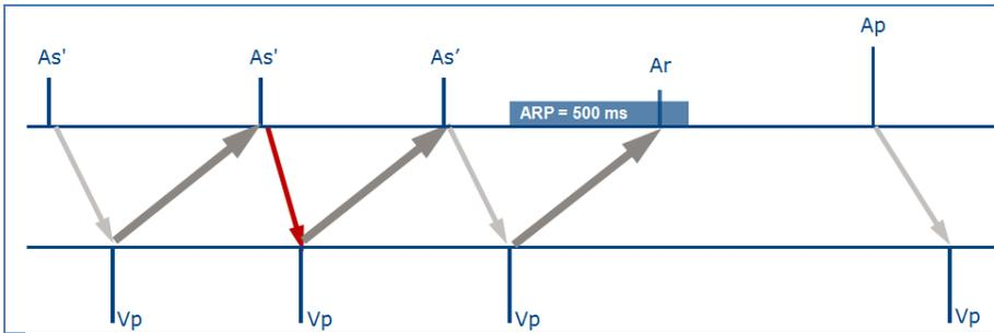
After a 50 ms AV delay shortening (in red), the stability criterion is still met (i.e.  $D[Vp-As'] < 15$  ms): the device confirms the PMT and applies the ARP on the next ventricular pacing to terminate the PMT.
