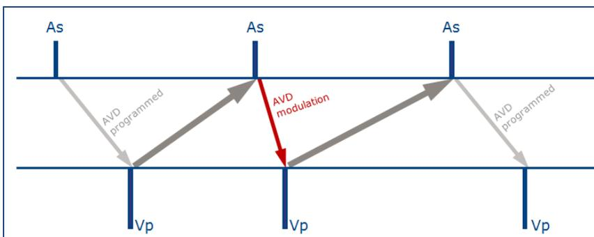
*Sinus tachycardia confirmation: After AV delay shortening (in red), the following [Vp-As] interval is different from the previous ones: the device diagnoses a sinus tachycardia*
