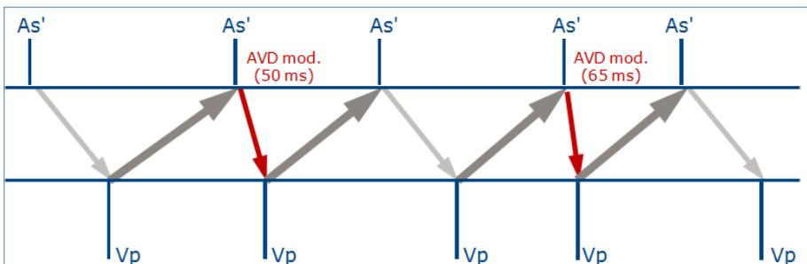
*In this example the strong stability criterion is met, therefore a 50 ms AVD modulation is applied (first red arrow). On the following [Vp-As] interval the weak stability criterion is met, therefore the device cannot conclude: sinus rhythm or PMT? A second AVD modulation (now 65 ms) is applied (second red arrow) to conclude. The strong stability criterion is met: PMT is confirmed.*
