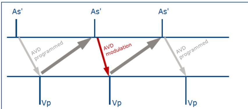
*PMT confirmation: After AV delay shortening (in red), the following [Vp-As] interval is stable: the device confirms the PMT*
