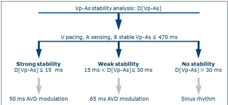
*PMT suspicion phase on 8 cycles: the device measures the retrograde conduction time (Vp-As) and enters in PMT suspicion if the Vp-As intervals are short ( $\leq 470$  ms) and stable ( $\pm 30$  ms)*
