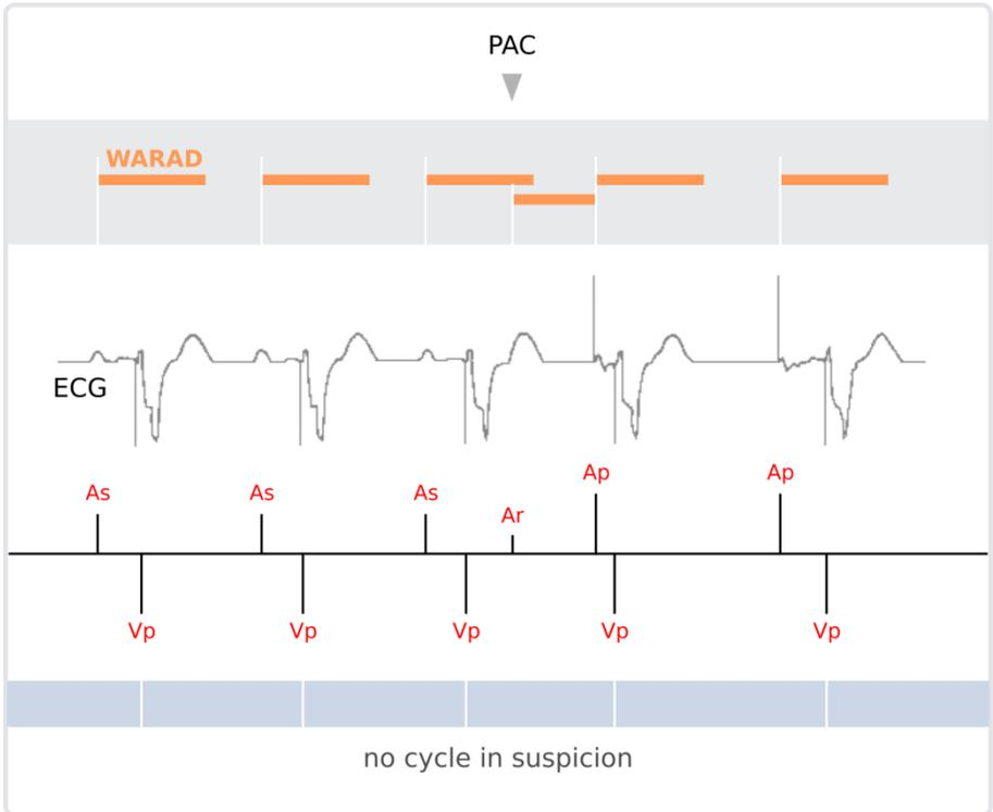
After sensing the PAC, the ventricular cycle ends with an atrial pacing so it is not considered as a cycle in suspicion of atrial arrhythmia.
