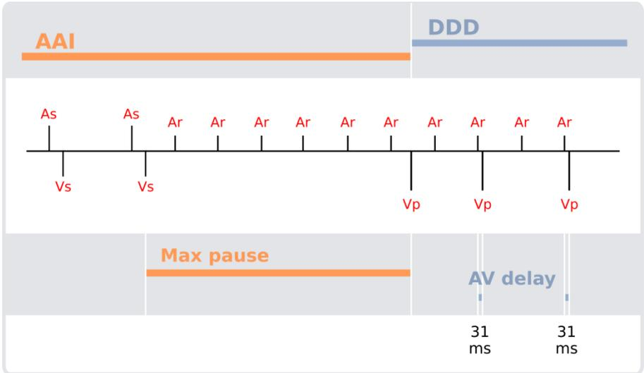
When the atrial arrhythmia is not conducted to the ventricles the device switches first from AAI to DDD mode on the Pause criterion. Then it will switch to DDI mode following one of the Fallback Mode Switch criteria.
