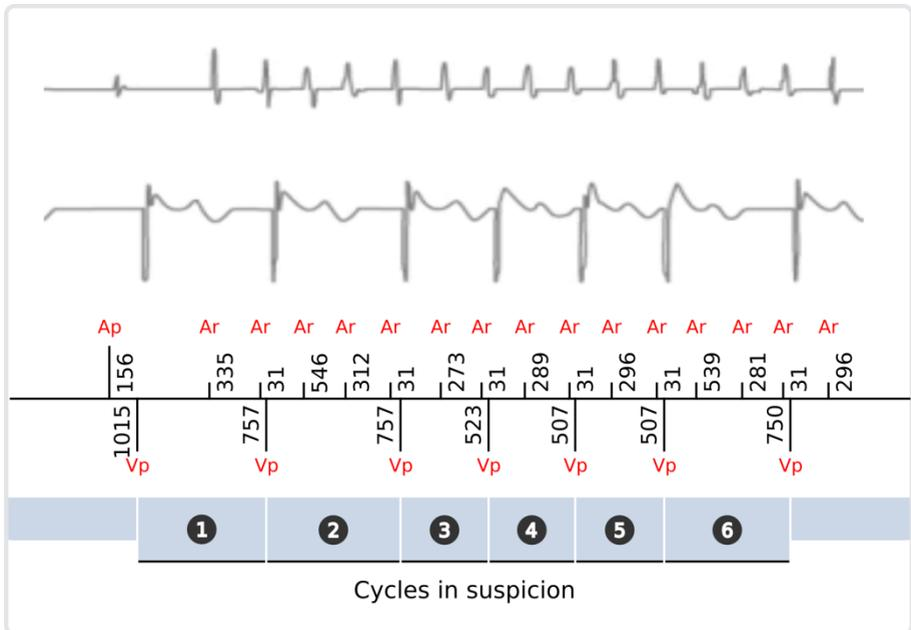
In this example we can see the onset of an atrial arrhythmia: ventricular cycles containing two or three PACs are considered as cycles in suspicion. Note that during the suspicion phase, the ventricular cycles are at least 500 ms (max ventricular rate: 120 bpm). Refer to the WARAD Tech Corner for more details on the ventricular rate management
