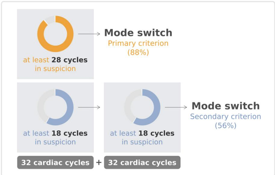
*Suspicion of sustained atrial arrhythmia: mode switch, with automatic management of atrial loss of atrial sensing during atrial arrhythmia*
