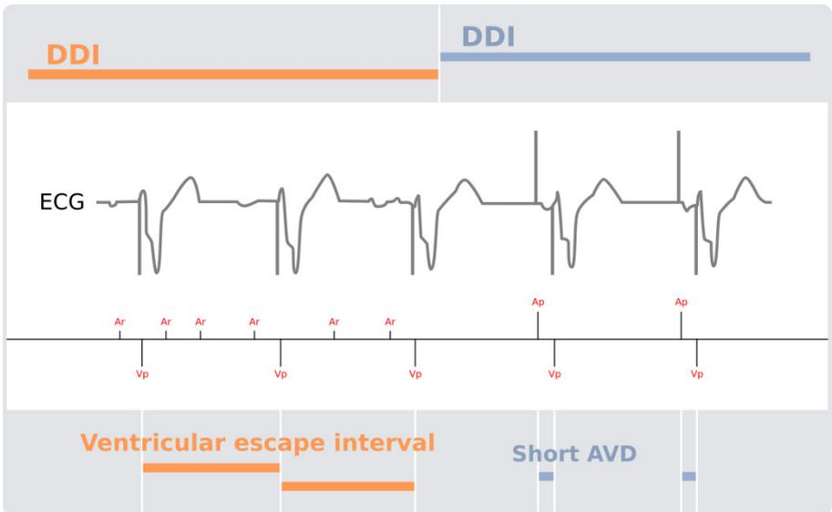
At the end of atrial arrhythmia, the device immediately paces the atrium applying a short AV delay for 24 cardiac cycles.
