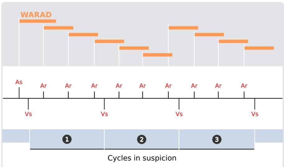
*Ar events are not considered as blocked atrial events. In the event of a conducted atrial arrhythmia, the device will switch directly from AAI to DDI mode following one of the Fallback Mode Switch criteria.*
