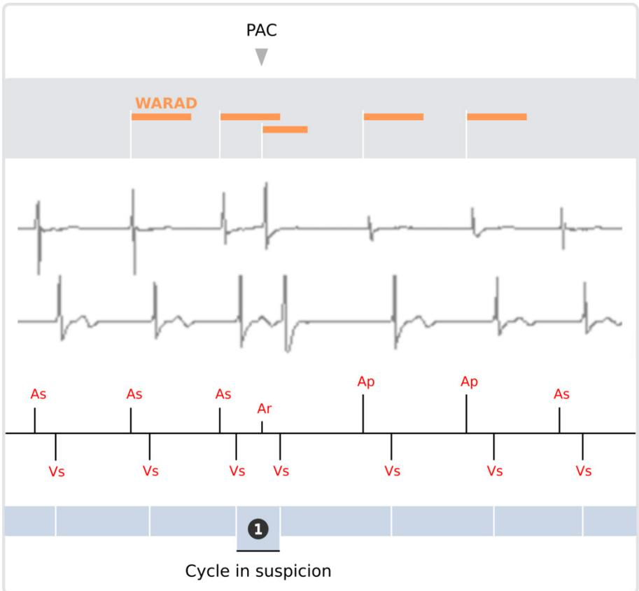
After sensing the PAC, the ventricular cycle does not end with atrial pacing so it is considered as a cycle in suspicion of atrial arrhythmia. All other cycles are not in suspicion since they do not contain any PAC.
