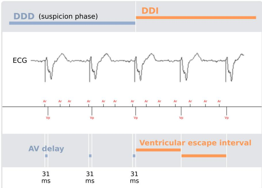
As long as the device is in the suspicion phase, it applies the 31 ms AV delay and limits the ventricular pacing rate at 120 bpm. Once it switches into DDI mode, it progressively paces the ventricles at the basic rate (or sensor rate).
